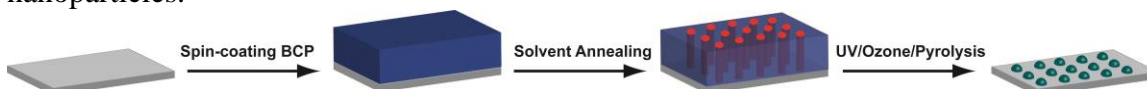
Scheme 4.1. Preparation of ordered BCP films and their template synthesis of iron oxide nanoparticles.
